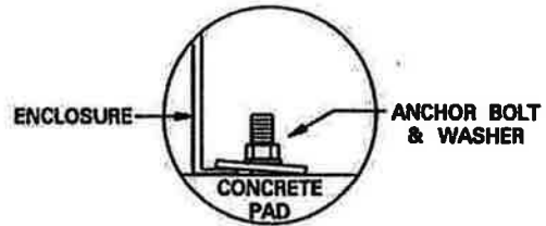
ANCHOR BOLT DETAIL
